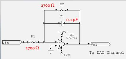
Set  $R_1=R_2$  to give gain of -1
